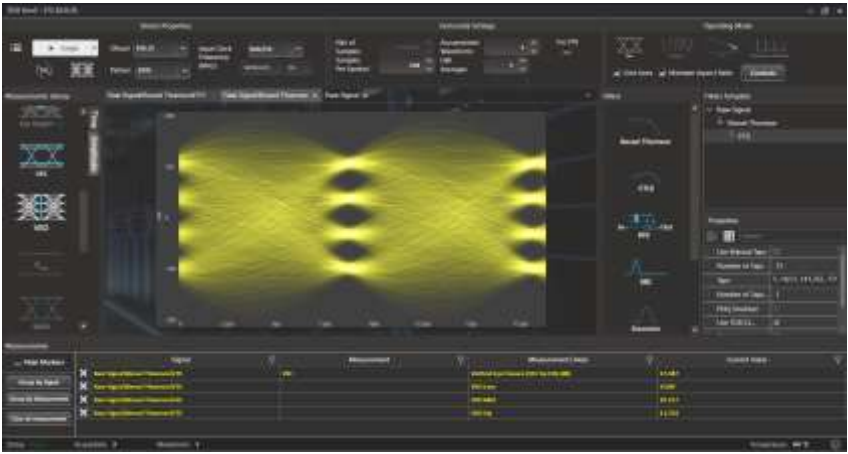
Figure 6: 112 GBaud (or 224Gbps) Electrical Eye Diagram with BT4 and 21 Taps FFE
